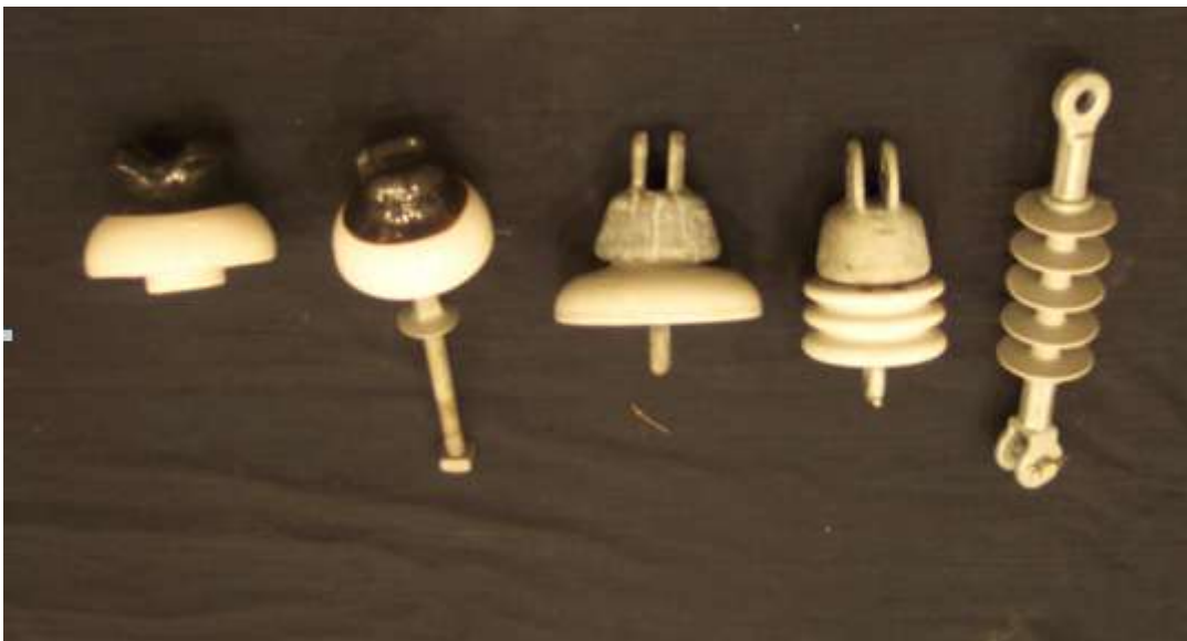
Figure 7-25. Insulators tested. This has two views of tested insulators, from the left: Pin type: ANSI 55-4, ANSI 55-3; Suspension type: ANSI 52-1, ANSI 52-9; 15 kV Polymer.
