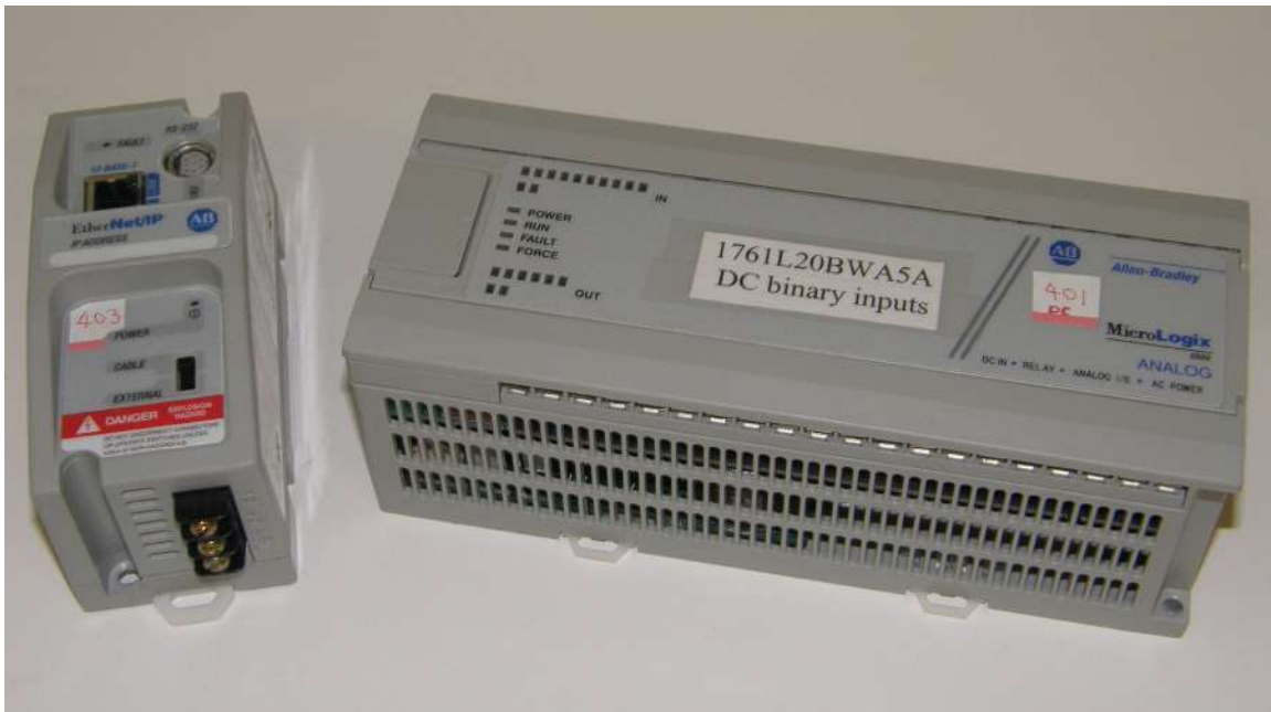
Figure 7-15. The Allen-Bradley MicroLogix 1000 PLC. The PLC, the unit on the right, has analog and binary I/O ports. Its communications is handled by the 1761-NET-ENI unit shown on the left.
