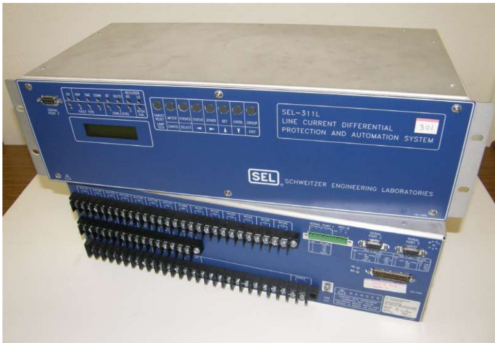
Figure 7-10. Modern relay unit. This is the SEL-311L (front view on top, back view on the bottom).
