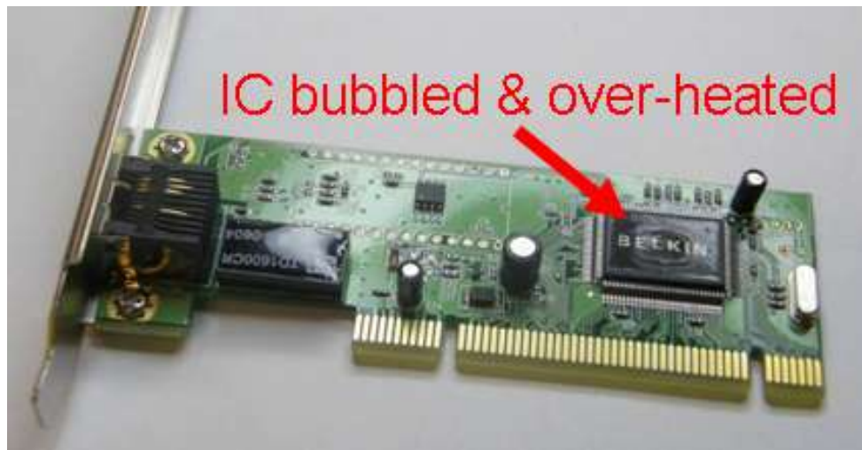
Figure 6-3. The result of pulse testing – IC damage. The IC lid, normally flat, has bubbled, and is discolored from over-heating.
