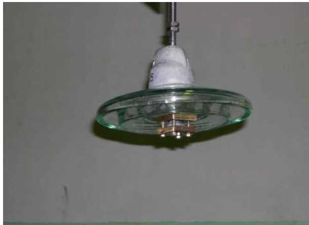
Figure 7-26. Suspension glass insulator for 10 kV power line.
