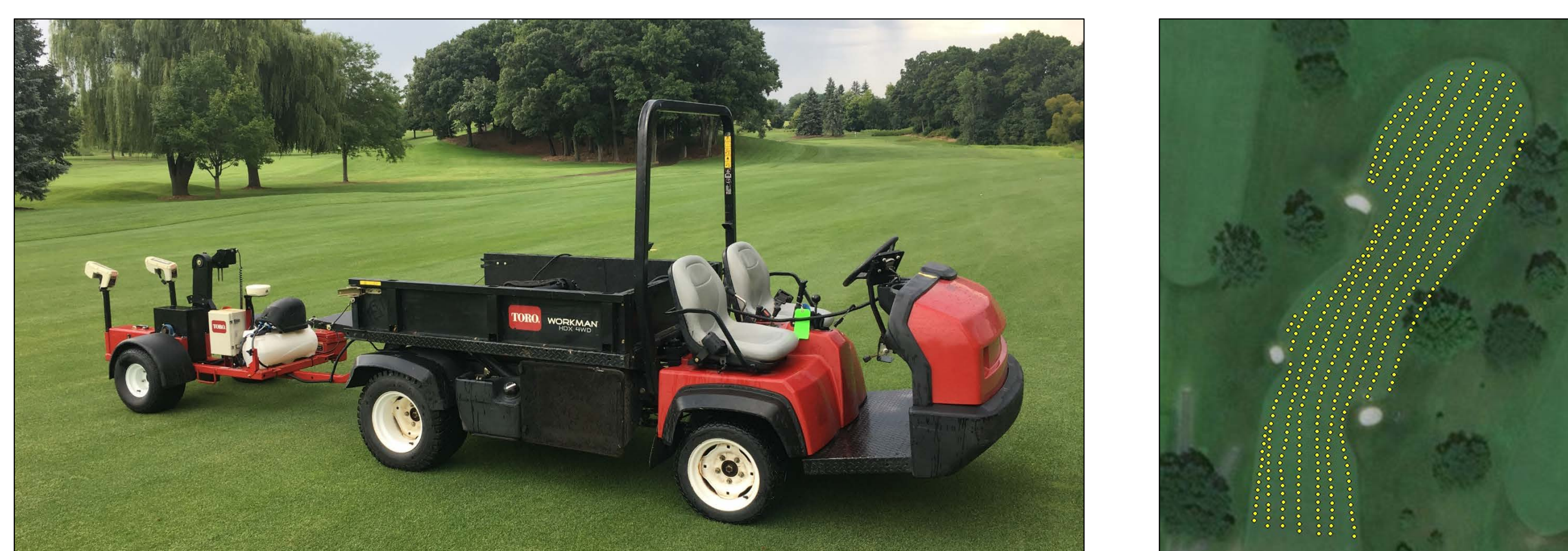
Figure 1. The PS6000 attached to the hitch of a utility vehicle (left) and an example of georeferenced data points from one fairway (right). Each yellow point represents a measurement location.
