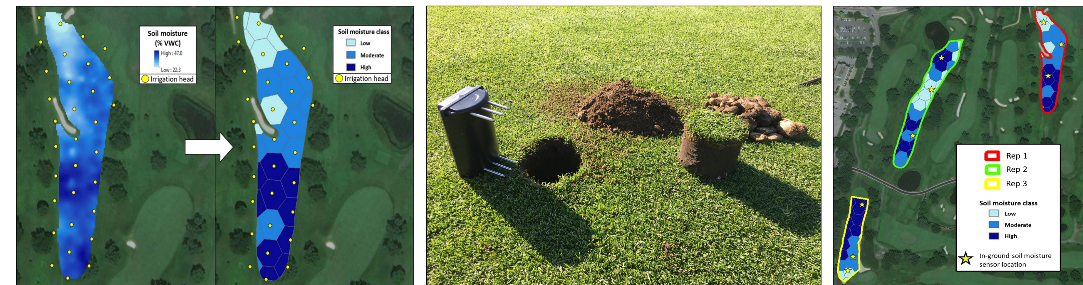
Figure 3. The irrigation management zone delineation and classification process (left), an in-ground SMS (center), and in-ground SMS locations within each fairway receiving the SMS-based treatment (right). "High," "moderate," and "low" soil moisture classes represent the wettest, average, and driest areas of a fairway, respectively.
