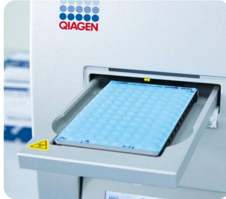
QIAGEN's QIAcuity digital PCR system is used to analyze target sequences
