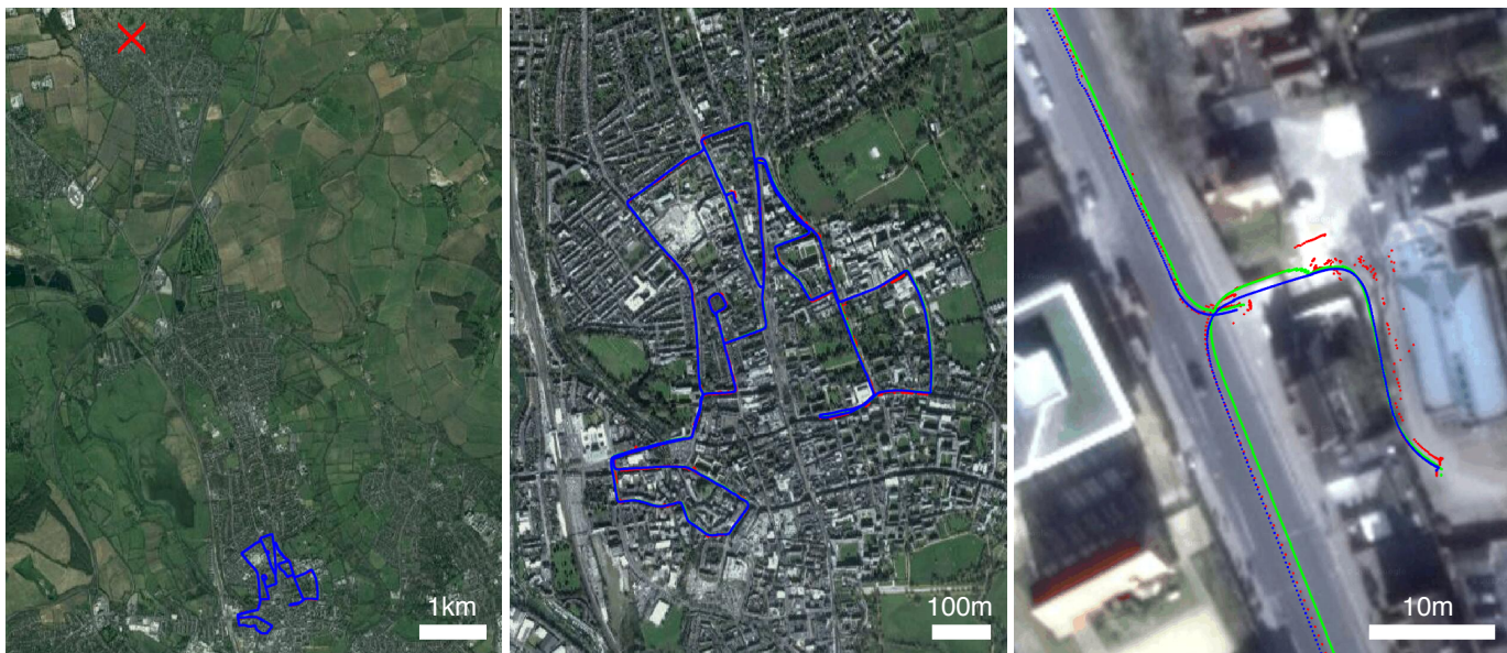
Figure 1. RTK ground truth for a single traversal from the Oxford RobotCar Dataset . Left: The GNSS base station location, shown with the red X, relative to the data collection route. Center: 80 traversals (72 released and 7 withheld) of the 10km route have been processed for localisation ground truth. Right: Quality of the RTK position solution (blue) compared to the GPS-only (red) and GPS-inertial (green). A subset of seven RTK ground truth files have been withheld to form a planned localisation benchmark which is under development.
