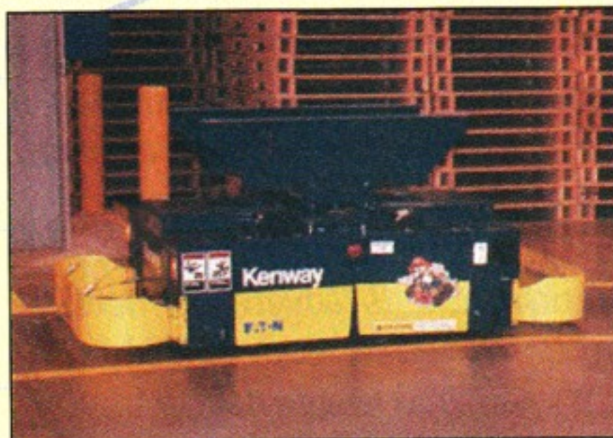
This wire-guided robot runs on its own and plugs itself in if its battery is low.
