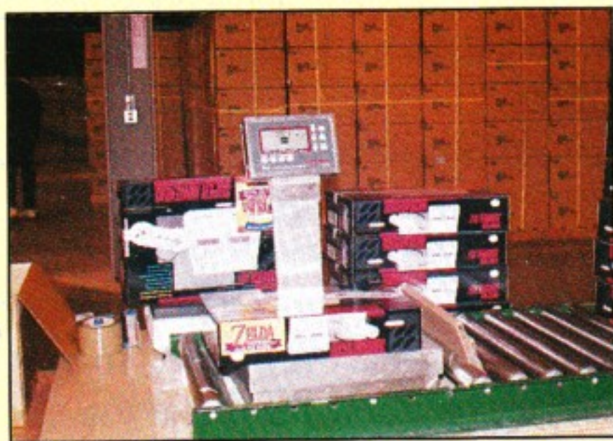
This scale is so sensitive that it can detect a missing manual from the box.
