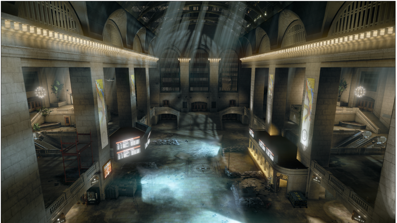
Figure 7: This scene contains many sources of geometric aliasing with low shading frequency, which are particularly well suited for SRAA. For instance, it is able to correctly reconstruct the brick structure along the roof, as well as the bent fence at the far end. The image has been reconstructed using 4 subsamples on an ordered grid to a target resolution of 1920 \times 1080 pixels in 2.5 ms. Scene courtesy of Crytek from Crysis 2 .
