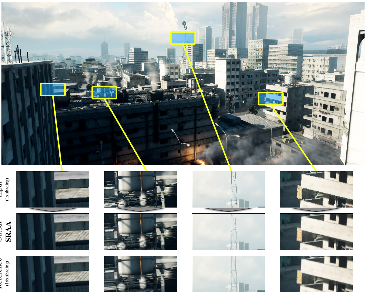
Figure 9: SRAA reconstructs subpixel edges while preserving sharp texture and shading features. The large image was processed by SRAA. The details compare the 1x input, the SRAA output, and the 16x shaded reference. Scene courtesy of DICE from the Frostbite 2 game engine. Zoom the electronic version of this paper to see pixel-scale detail. The reconstruction at the target resolution ( 1920 \times 1080 ) took 2.5 ms.
