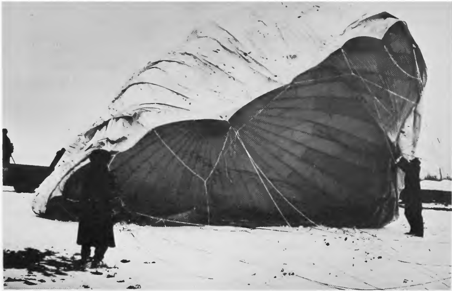
Figure 27. Wind catches a recovered balloon like a parachute. Note the arrangement of the gores on the lower surface with the relief valve in place. Photo taken on 23 February 1945. (29907 AC)
