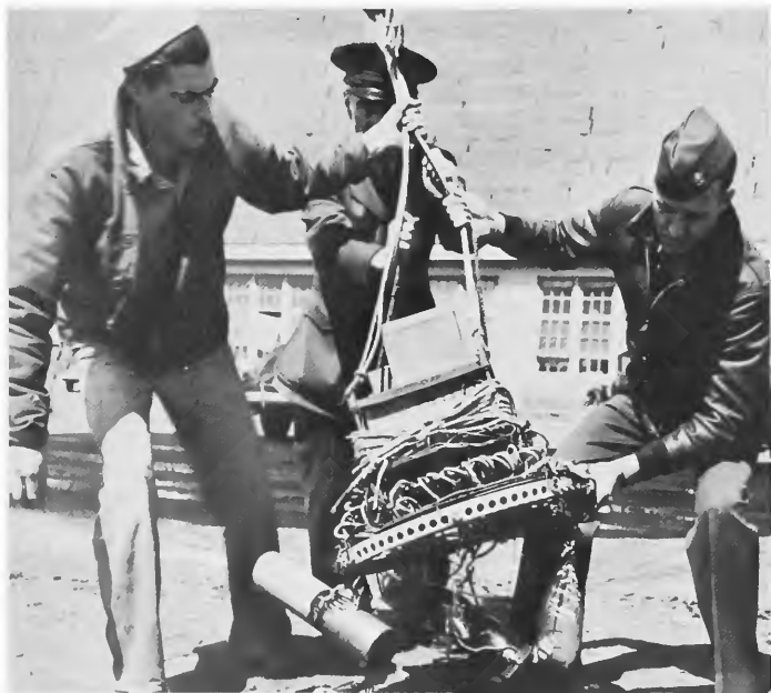
Figure 36. On the left periphery of the release ring is a 5 kg thermite incendiary bomb sometimes used as ballast in the last release stations prior to the dropping of the main bomb. (U.S. Navy photograph, 80-G-326355, in the National Archives)
