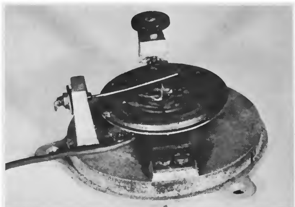
Figure 57. This aneroid marked with a triangle on its cap rendered the altitude-control device inoperative until the balloon initially ascended through 6,000 to 16,000 feet. This served as a safety against inadvertent release of explosives. (72-870)
