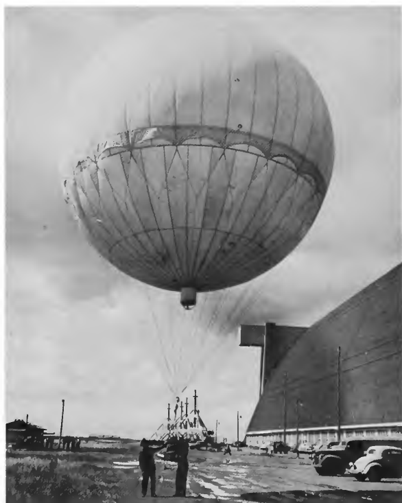
Figure 34. This inflated balloon shows the geometry of the many paper gores which make up the gas-proof envelope. Nineteen shroud lines attached to the cloth skirt carry the gondola. (U.S. Navy photograph, 80-G-326353, in the National Archives)
