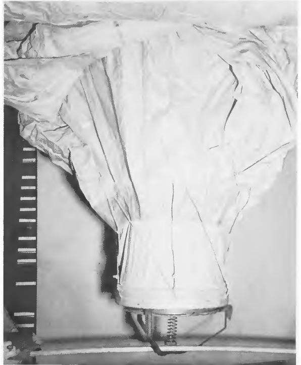
Figure 41. Gas relief valve glued in position at neck of envelope. This balloon was recovered near Holy Cross, Alberta, Canada, on 21 January 1945. (U.S. Army photograph, SC 237084)
