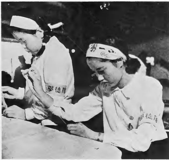
Figure 12. Great numbers of Japanese high-school girls were used in the delicate work of pasting and stitching the balloon envelope.
