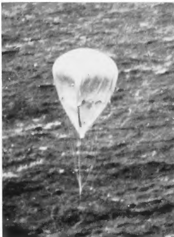
Figure 26. Partially inflated balloon, with its bomb load, in flight over the Pacific Ocean drifting toward the American continent. (U.S. Army photograph, SC 226132)
