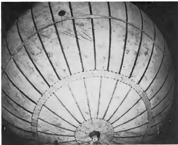
Figure 7. Imperial Japanese Navy’s balloon development consisted of a rubberized-silk envelope. Due to the weight, its payload was much less than the paper balloon developed by the army. (U.S. Air Force photograph, 30770).
