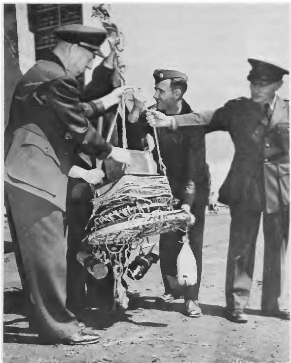
Figure 35. United States Navy personnel steady the ballast-dropping mechanism and bomb-carrying device. The main bomb is suspended in the center, while a ballast sandbag hangs at the right. (U.S. Navy photograph, 80-G-326354, in the National Archives)
