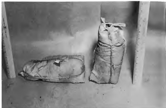
Figure 66. Thirty-two sandbags made up the ballast load for balloon altitude control. Individual weights were approximately seven pounds. (U.S. Army photograph, SC 237089)
