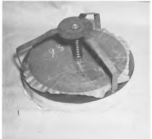
Figure 42. The gas relief valve, nineteen and one-half inches in diameter, was spring-loaded against a one-ounce-per-square-inch gas pressure. This valve, marked with a chalk number "93," was recovered at Marshall, Alaska, 23 December 1944. U.S. Army photograph, SC 237090)
