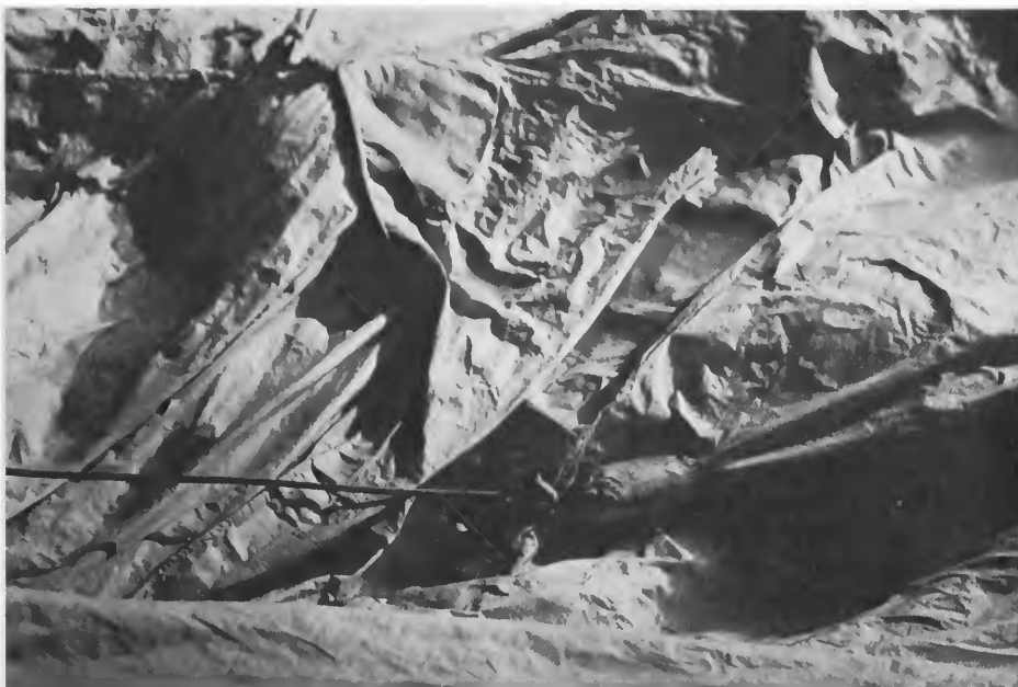
Figure 48. Close-up of the ignition charge attached to the side of the envelope and fuse leading to it. At the top left is a shroud line attached to the catenary band. (30781 AC)
