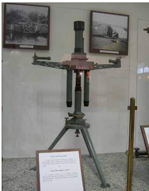
The Eötvös-Pekár and AUTERBAL balances in the Eötvös Loránd Memorial Exhibition. The telescope arms of the AUTERBAL can be detached from the balance. During surveying they are not used, but have a control function in instrument tests only.
