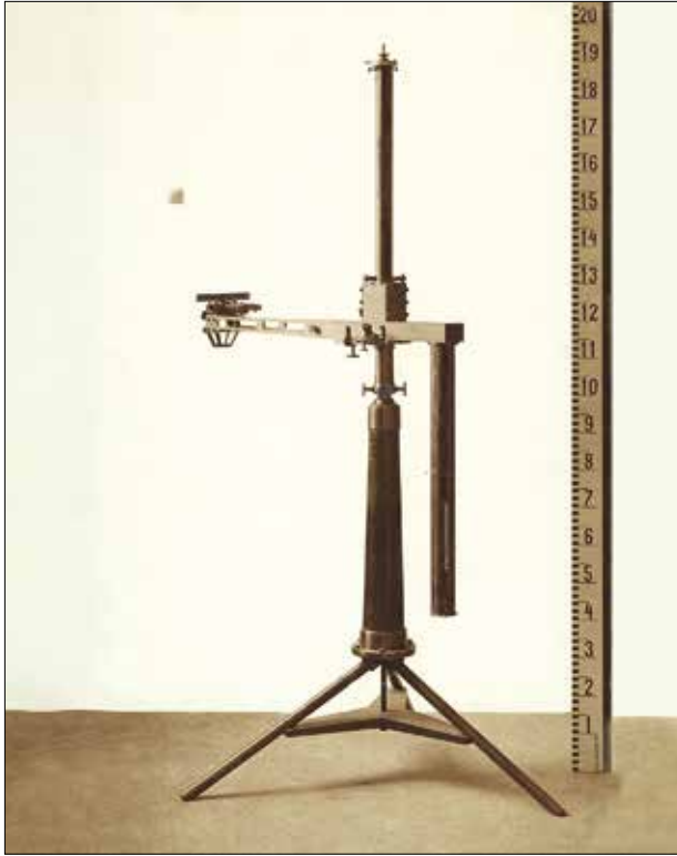
The so-called Balaton balance (a single Eötvös balance), shown in a paper by Eötvös, and the same instrument on display in the Eötvös Loránd Memorial Exhibition today
