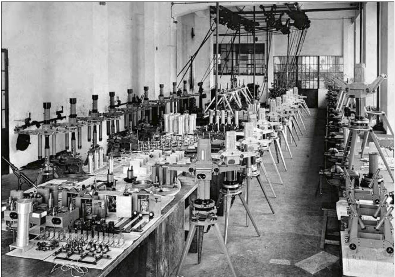
Eötvös-Pekár and AUTERBAL balances being assembled at the Süss factory in around 1930
