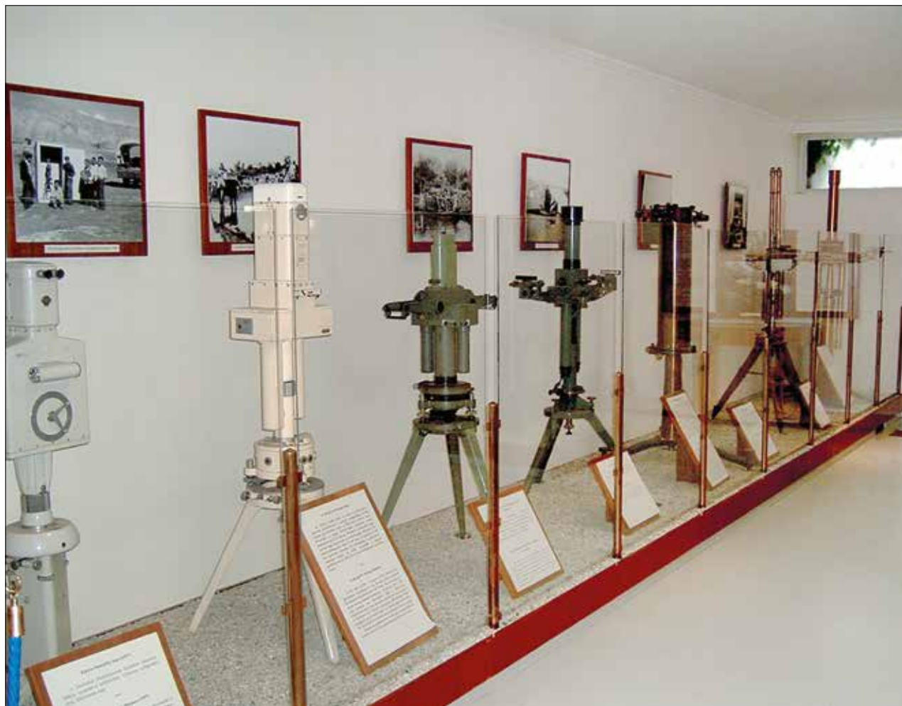
The stages of development of the Eötvös balance on display in the Eötvös Loránd Memorial Exhibition, from right to left: double large balance, double small balance, double balance with water cooling (which did not fulfil expectations), Eötvös-Pekár balance, AUTERBAL balance, E-54 balance, Eötvös-Szecsődy balance
