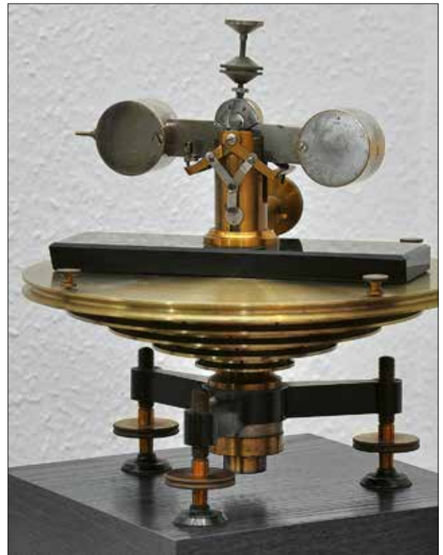
The Eötvös rotating seesaw, which measures the angular velocity of the Earth by exploiting the Coriolis effect. (The seesaw in the photo belongs to the Eötvös Loránd Memorial Collection, Budapest.)
