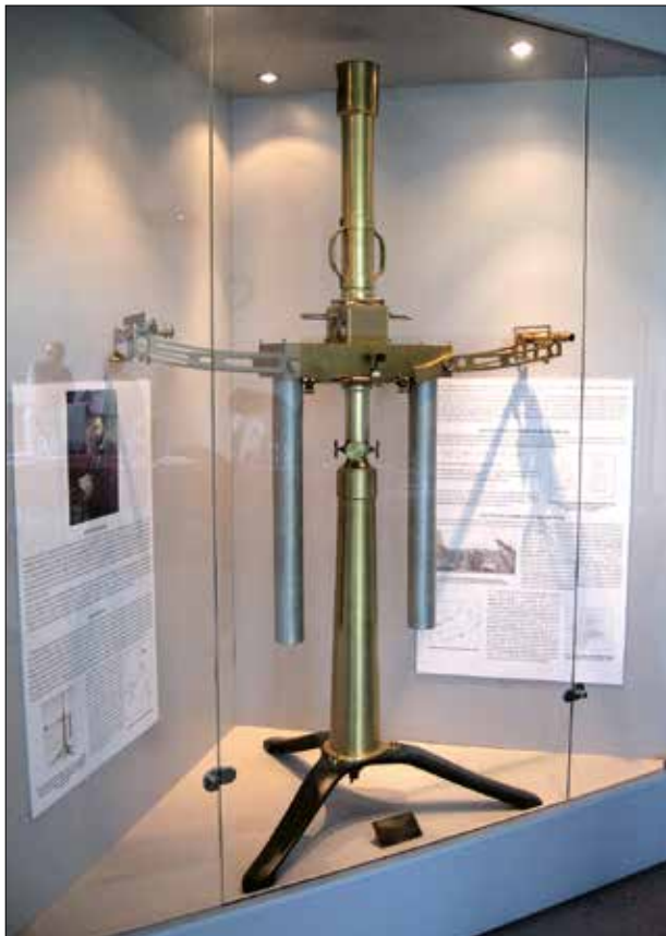
The prototype of the “double balance” (1902) on display in the Department of Geophysics at Miskolc University, and a “double small balance” (1908) in the Eötvös Loránd Memorial Exhibition
