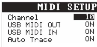
Strike the pad you desire to edit and then use the +/- or rotary button to find the option you wish to adjust. Pressing the return button then allows you to use the +/- or rotary button to adjust the settings.
