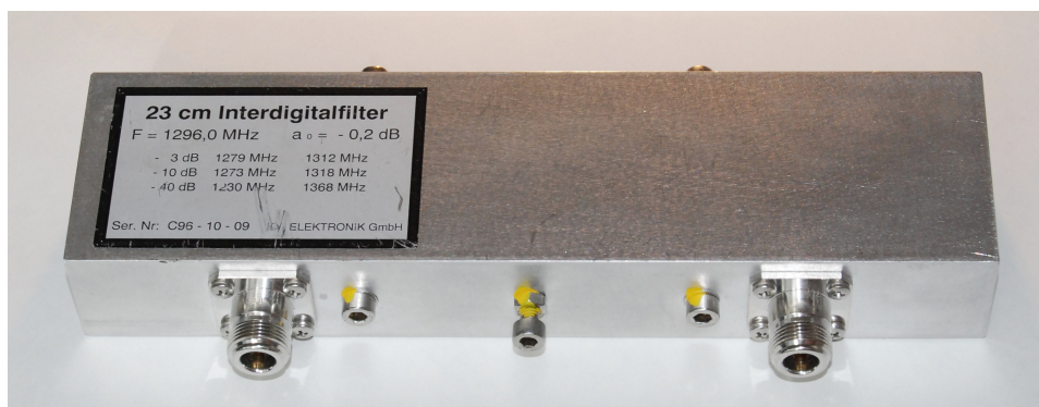
Figure 7.12 The interdigital BPF with a -3 dB bandwidth amounting to 33 MHz. The insertion loss is 0.2 dB at the 1296 MHz centre frequency.
