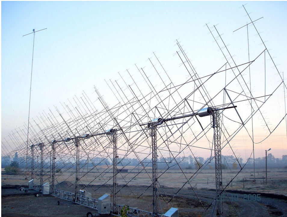
Figure 2.6 A 144 MHz EME antenna array belonging to Sam Dubovtsev (R7AB). The array consists of 64 crossed long-yagi antennas with 2 \times 15 elements each, yielding a total gain of about 34 dBi. Vertical or horizontal polarization can be chosen at the flick of a switch. Resting on several wheels the antenna has full azimuth as well as elevation control capability. (Courtesy of Sam Dubovtsev [46].)
