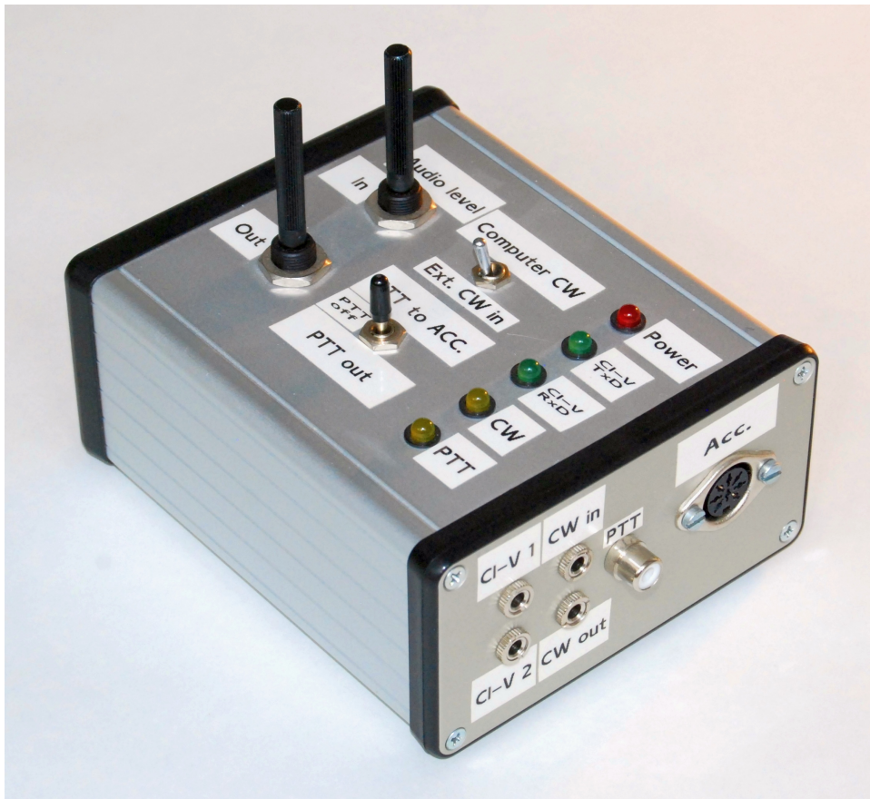
Figure 7.13 The audio and data interface, used for interfacing the computer to the rest of the system. The audio and serial port connectors are on the opposite side of the box.
