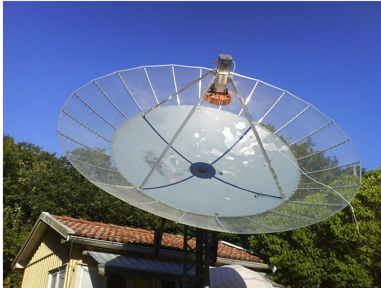
Figure 8.11 The 4 metre dish pointed straight at the Sun during a Y-factor and drift-scan measurement. The antenna was not moved between the hot and cold measurements. Notice how the shadow of the feed horn is in the middle of the reflector. At the time of this photo, the measured noise level was at its maximum.
