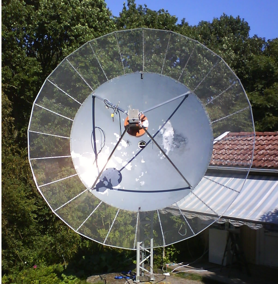
Figure 7.2 The extended prime focus parabolic dish. The dish diameter is solid out to 2.7 metres and extended to 4.0 metres using 24 aluminium ribs and meshed wire netting, resulting in f/D = 0.30 . Also shown is the septum polarized feed horn and the four accompanying support struts.
