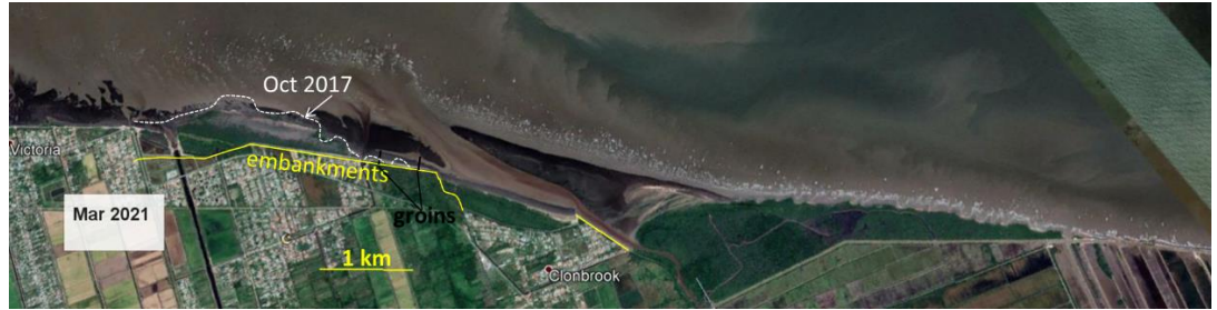
Figure 8.2 Development of natural grey-green infrastructure in front of Clonbrook, close to the left bank of the Mahaica River (Google Earth images).
