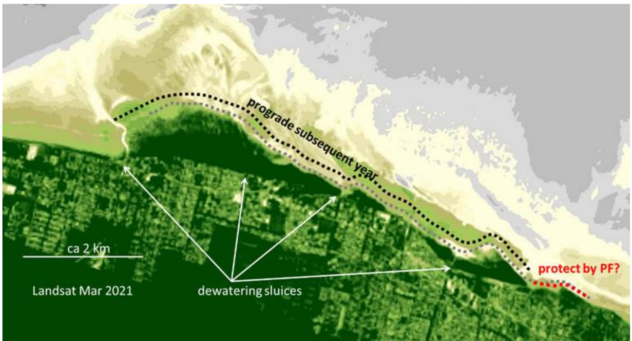
Figure 13. Schematic of deployment of MudBank Motor concept along Chateau Margot mudbank consisting of Sediment Trapping Units on the intertidal mudflats behind the mudbank and protecting permeable bamboo fences along the tail of the mudbank
