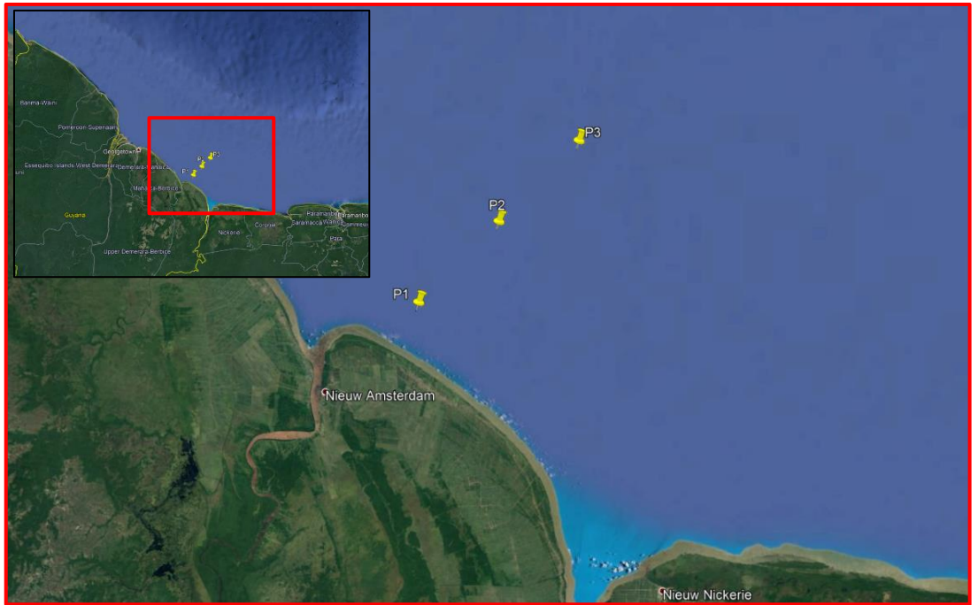
Figure 12.1 Location of the transect at which the ERA5 wave data was extracted, in front of the coast of Nieuw-Amsterdam at locations 10 km offshore (P1), 30 km offshore (P2) and 50 km offshore (P3). The smaller panel (top left) provides a large-scale perspective of the Guyana coastline, and the larger panel (red box) provides a zoom near Nieuw-Amsterdam.
