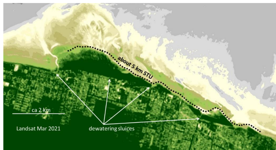
Figure 13.4 False-colour Landsat satellite image of Guyana coastal zone around Georgetown and indicative location for STU-construction.
