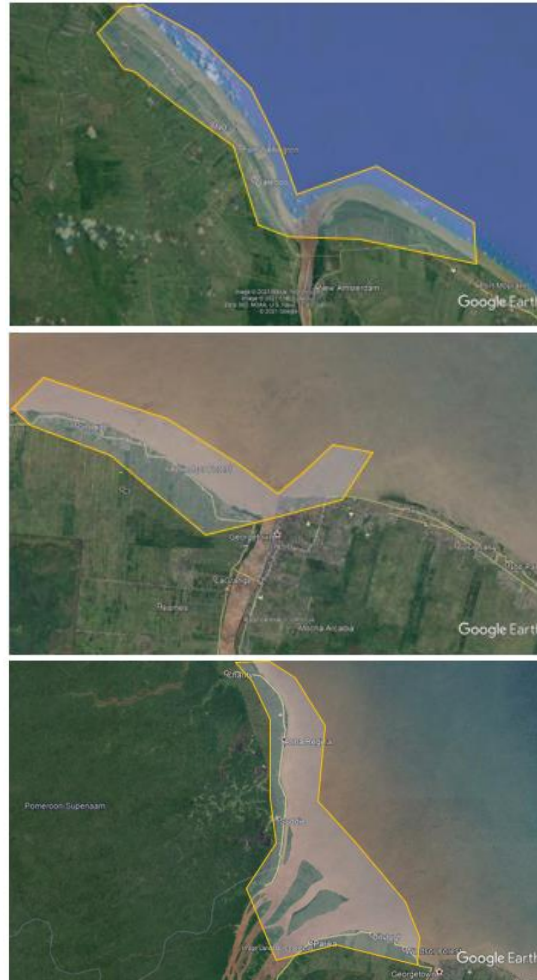
Figure 14.2 Schematic of the likely spatial extent and reach of the freshwater discharge from the main rivers in Guyana, (top) the Berbice River, (middle) the Demerara River and (bottom) The Essequibo River .
