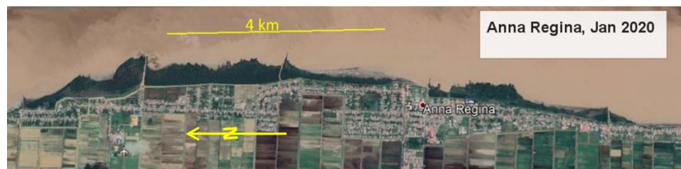
Figure 7.4 Mangrove development in between groynes near Anna Regina, left bank of the mouth of the Essequibo River.
