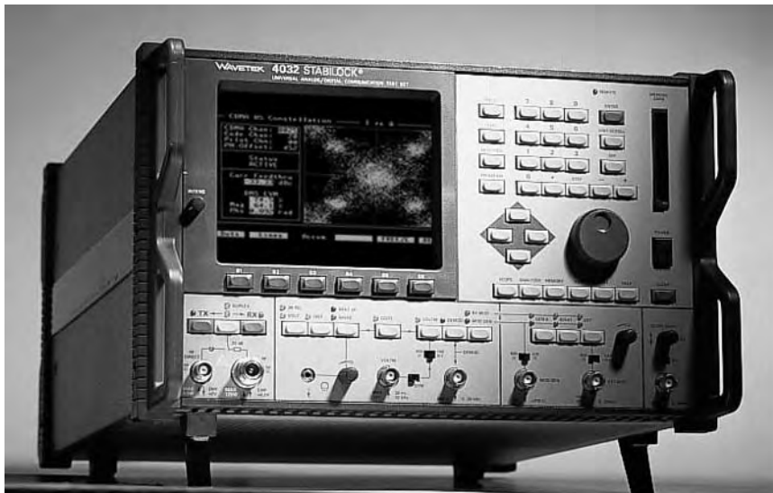
Figure 10.9 A typical communications test set, like this one, incorporates several instruments in a compact package, saving the technician from carrying several instruments to hard to reach sites or using up too much bench space.
