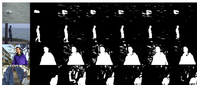
Figure 4. Comparison of results from different algorithms. First Column - Original images; Second Column - Ground Truth; Third Column - OriginalMoG; Fourth Column - Eigenbackground [14]; Fifth Column - ViBe [15]; Sixth Column - MGMUM [16]; Seventh Column - SpatialMoG
