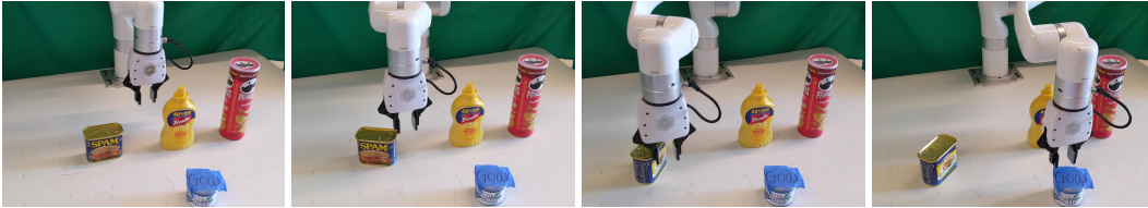
Figure 5: We demonstrate successful execution of the LAPP-TrajOpt path planning algorithm in the real-robot system. A path to the goal, specified by the blue jar, is blocked by diverse objects on the table, so the robot needs to collide with some object. We inform which object is safe and desired to collide using the language prompts: “pringles, cheezit”, “pringles”, and “spam”, respectively.
