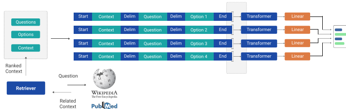
Figure 7: The Retriever+Reader Pipeline for Open-Domain Question Answering system used in our experiments. Dense passage retrieval (Karpukhin et al., 2020) and PubMedBERT (Gu et al., 2022) are used to evaluate Wikipedia and PubMed as knowledge bases respectively, while different transformer models (explained in section 5) as reader models.
