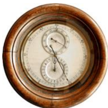
The Hipp Observatory (slave dial) clock from Peyer Favarger & Co. was controlled by the Riefler slave clock in the master clock vault and was visible to the astronomer operating the Meridian Circle Telescope. Photo by L. Hite
