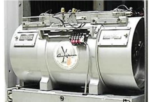
An Audichron talking clock announced the time, hour, and minute. Image from Wikipedia
