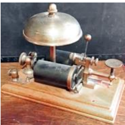
This telegraphy activated fire and time bell sounded at the Milwaukee (Wisconsin) Fire Department. Image from Old Fire Stuff
