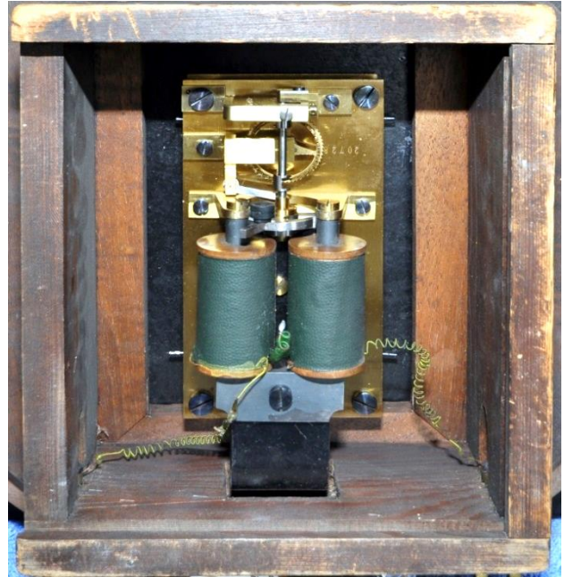
These images feature the Hipp Observatory (slave dial) clock working details.
