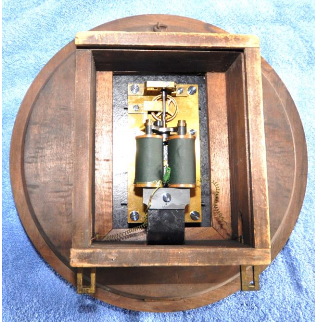
These images feature the Hipp Observatory (slave dial) clock working details.
