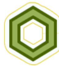
Buffering a polygon with one interior ring
