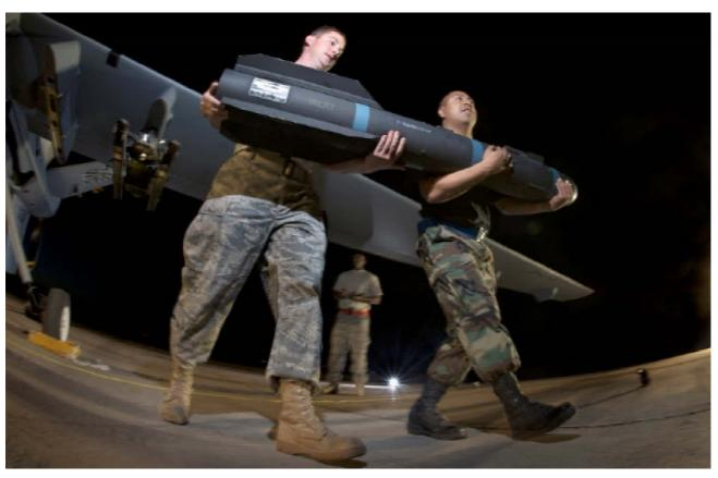
Armourers unload an AGM-114 Hellfire Missile from a MQ-9 Reaper. Photo courtesy DoD.
