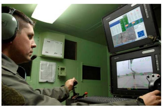
Inside the Ground Control Station of an MQ-1 Predator. Photo courtesy DoD.
