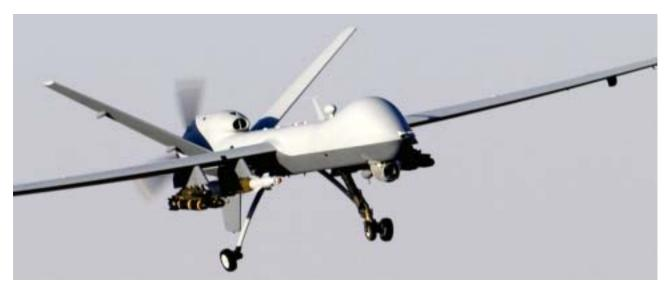
An Armed ISR UAV: General Atomics Aeronautical Systems MQ-9 Reaper. *Photo courtesy DoD*.
