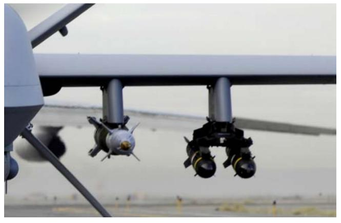
Two AGM-114 Hellfire Missiles and a GBU-12 Paveway II Laser Guided Bomb under the wing of a MQ-9 Reaper. *Photo courtesy DoD*.
