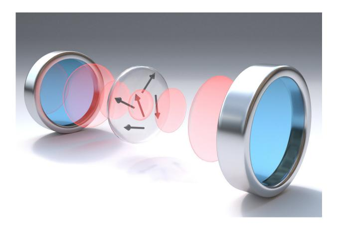
The Garching quantum modem: The crystal disk with the quantum bits of erbium atoms (arrows) is in the middle, the back and forth reflected infrared light is indicated by the red disks. Credit: Christoph Hohmann (MCQST)
