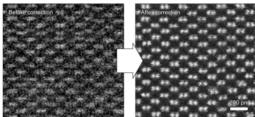
**Fig. 4.9.2.** Scanning TEM micrograph of silicon “dumbbells” before and after automatic aberration correction. *Source:* Inada H, *et al.* High-speed and sensitive x-ray analysis system with automated aberration correction scanning transmission electron microscope. *Applied Microscopy*. 2015;45(1):1–8. *Credit:* Creative Commons CC BY-NC 3.0.
