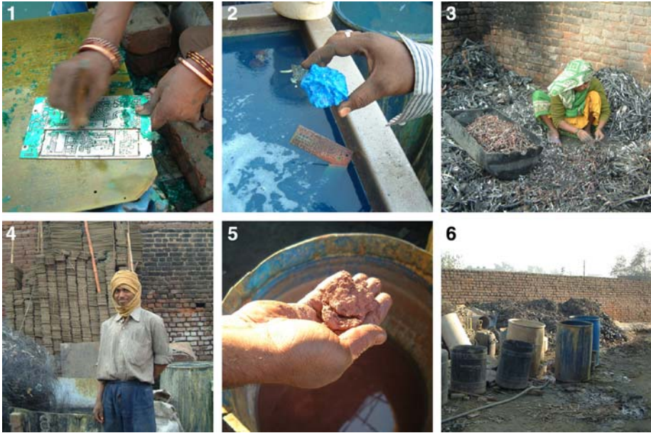
Fig. 4 Extraction of copper from printed wiring boards (PWBs): (1) manually removing varnish, (2) recovering copper-sulphate after submerging PWBs for 12 h into sulphuric acid by boiling off H_2O using PWB residues as a fuel, (3) manually segregating the copper layer and glass fibres after burning multi-layer PWBs (as they are resistant to the acid), (4) scrap iron is added to the remaining liquid to react with the dissolved copper, (5) fallen out copper slime is a third product bringing the total to 1–2 t of copper per month, (6) such an enterprise creates about 12 jobs, however at high-external costs. Source Widmer et al. (2005)
