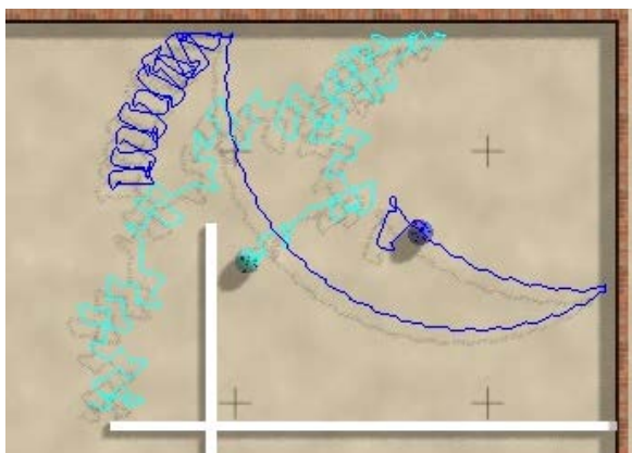
Fig. 3. Two color-coded copies of the sphere robot exploring a maze. The motions can be classified as strongly chaotic for the cyan robot and as partially predictable chaos for the blue robot [5]. The blue robot switches to another locomotion mode after colliding with the wall. The resulting radius of the circular mode is, however, too large for the maze and it can follow it hence only transiently. [video]
