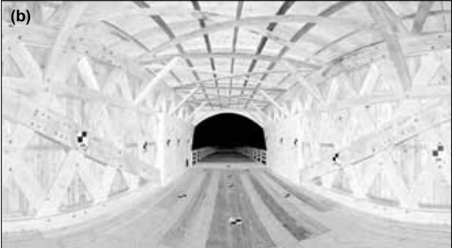
Figure 24. Planar views of a single laser scan of the Roseman Bridge (NRR).
