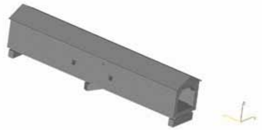
Figure 38. A 3D isometric image of the Zumbrota Bridge used to produce a 1/100th model using selective laser sintering rapid prototyping equipment.
