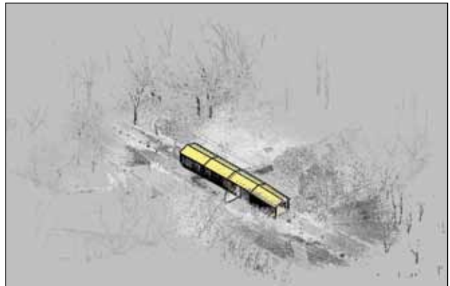
Figure 11. 3D AutoCAD image of the Cedarburg Bridge embedded in point cloud data (SightLine, LLC).
