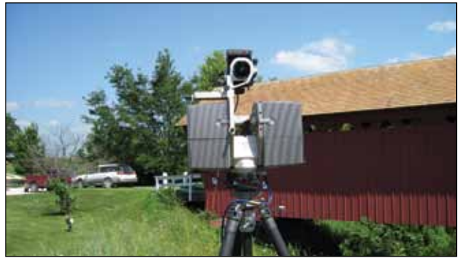
Figure 9. A FARO laser scanner used to scan a historic covered bridge.
