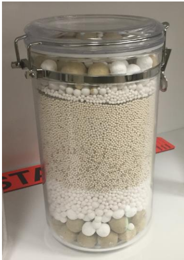
Sample packing of catalyst on top of supports Model prepared by Enterprise Products
