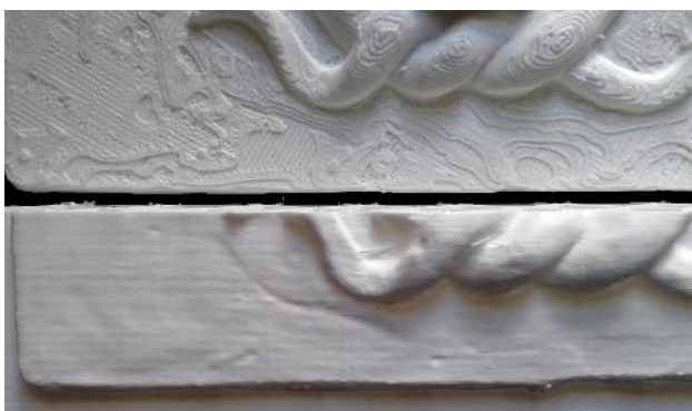
Figure 9. The Medusa mask; up side, horizontal printing; down side, vertical printing
