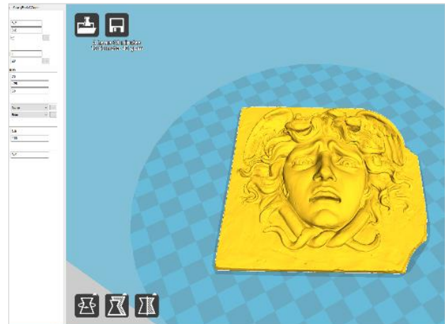
Figure 5. The main screen of Cura; the Medusa mask, horizontal position, normal view mode
