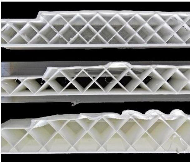
Figure 12. Three prototypes of the Medusa mask, vertical position. Different settings of fill density (10-15-20 %).
