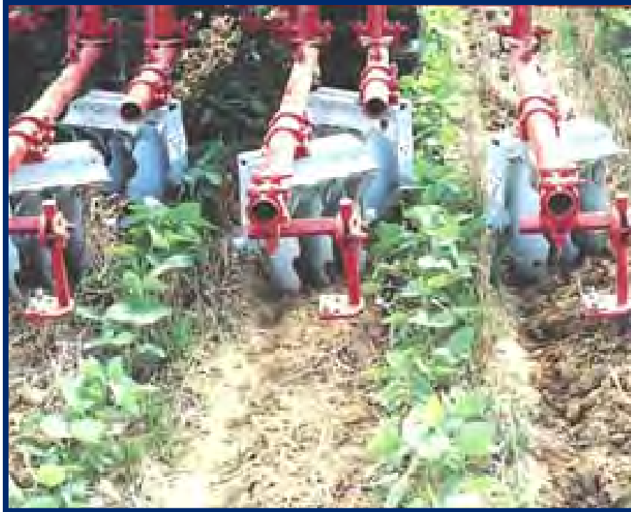
A gang of Lilliston cultivators used in double passes to manage weeds early in a potato crop.
