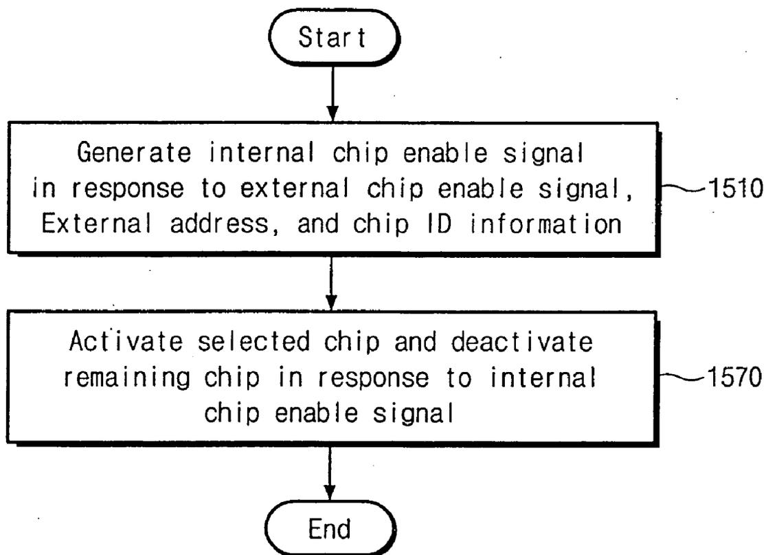
**LOW POWER MULTI-CHIP SEMICONDUCTOR MEMORY DEVICE AND CHIP ENABLE METHOD THEREOF**
