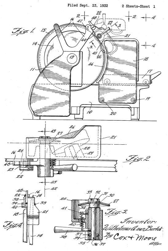
SLICING MACHINE KNIFE SHARPENER
