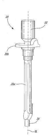
(57) Abstract: A method and a pre-shaped workpiece (20) for making at least a portion of a gas turbine fuel nozzle (20') are disclosed having opposed gripping tabs (22, 24) which can be secured to machine tool holders (32, 34) during manufacturing by a machine tool (30).
