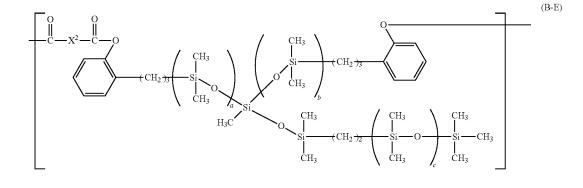
In the formula (B-E), X<sup>2</sup> represents a m-phenylene group, a p-phenylene group, or a divalent group obtained by bonding two p-phenylene groups through an oxygen atom.
