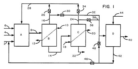
The present invention is directed to a process for producing oxo products, and more particularly to a process in which propylene, carbon monoxide and hydrogen are reacted in the presence of a suitable catalyst to produce oxo products, such as butyraldehyde and n-butyl alcohol, and unreacted propylene is recycled to the reactor.
