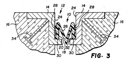
has spring means such as spring wire embedded within the joint-seal strip. The spring means expands the web member and urges the flange portions in the direction of the arrows shown in FIG. 2 into sealing engagement with the abutments when the seal strip is compressed
