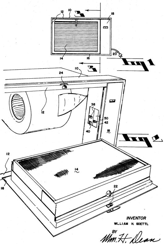
ELECTROSTATIC AIR CLEANER AND CONTROL MEANS THEREFOR
