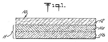
THROUGH BONDED BY POLYVINYL ALCOHOLAND POLYACRYLIC ACID REACTED IN SITU
