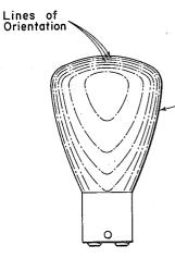
Non-crystalline molecular coating of individually oriented molecules of light-polarizing substance.
