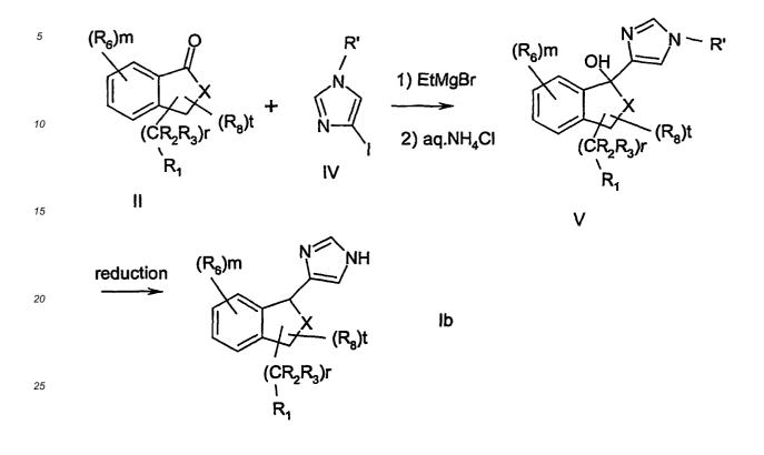
wherein X,  $R_1$  to  $R_3$ ,  $R_6$  and  $R_8$  m, r and t are as defined above and R' is a conventional protecting group for =NH in the imidazole ring, e.g. benzyl, trityl (-CPh<sub>3</sub>) or SO<sub>2</sub>NMe<sub>2</sub>.
