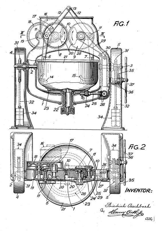
KNEADING AND MIXING MACHINE, PARTICULARLY FOR PASTE LIKE GOODS
