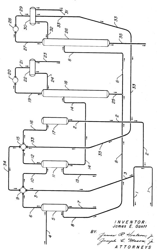
3,437,708 SEPARATION PROCESS FOR ALKYLATED AROMATIC COMPOUNDS AND OLEFINIC OLIGOMERIZATON PRODUCTS
