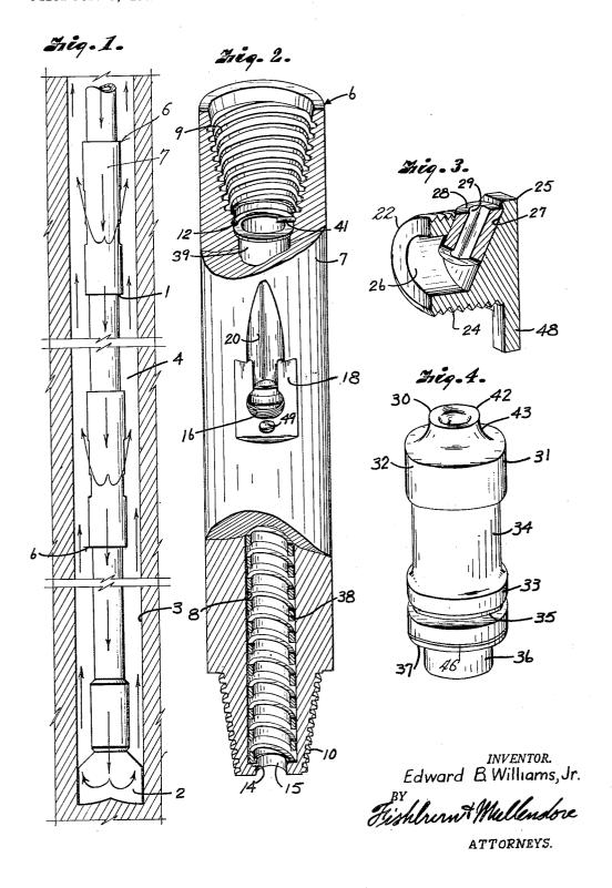
JETTING DEVICE FOR ROTARY DRILLING APPARATUS
