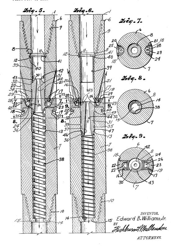
JETTING DEVICE FOR ROTARY DRILLING APPARATUS
