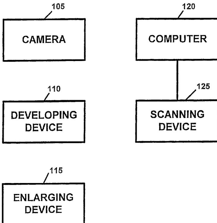
(57) Abstract: An apparatus and a method for producing a digital image, which includes a device for generating a digital signal file from a print film image (125) and a processor for processing the digital signal file and for generating an image file (120). The processor generates a first signal file from the digital signal file (120). The processor processes the first signal file and generates the image file (120).
