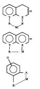
wherein X,Y,R,R', A, B, and G are as hereinbefore described, and M is a metal selected from the group con- 35 sisting of Cr, Al, Zn, Ti, Ta, Ni, Cu, Ga, As and alloys thereof.
