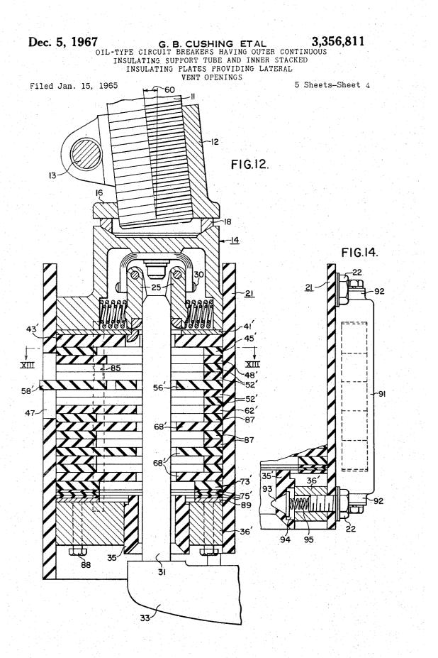
Dec. 5, 1967 G. B. CUSHING ETAL OIL-TYPE CIRCUIT BREAKERS HAVING OUTER CONTINUOUS INSULATING SUPPORT TUBE AND INNER STACKED INSULATING PLATES PROVIDING LATERAL VENT OPENINGS Filed Jan. 15, 1965 5 Sheets-Sheet 5
