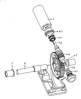
(57) Abstract: The invention is related to an independent power-train used to set the torque speed received from a drive motor or similar drive sources.
