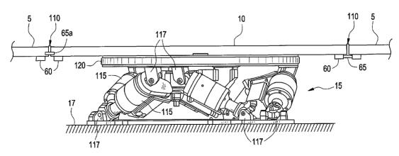
(57) Abstract: An amusement ride has a track (5) defining a ride vehicle path (100) with a section of the track (10) that can be decoupled from the main track and is subsequently movable on or about up to three axes with between one and six independent degrees of freedom.
