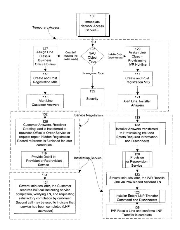
Figure 3 Immediate Network Access Service
