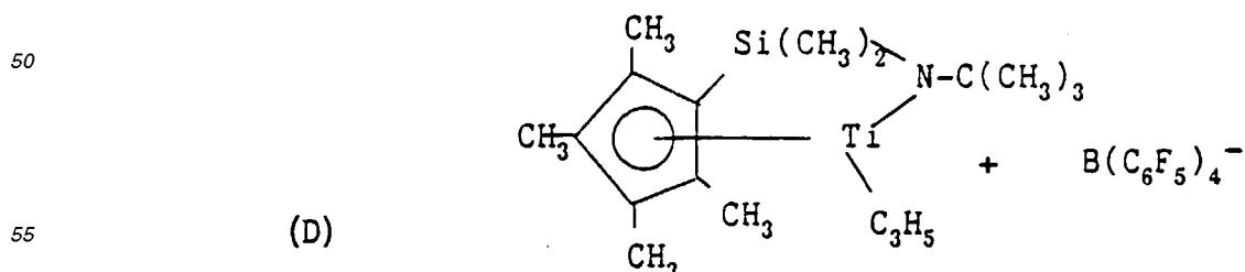
The reaction conditions of Example 1 were substantially repeated using equal molar amounts of the above reduced metal derivative and ferrocenium tetrakis-perfluorophenyl borate as the anionic oxidizer to cause metal center oxidation.
