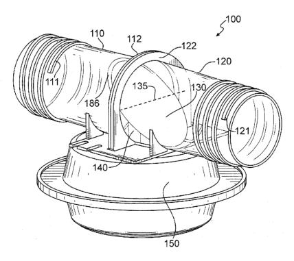
(57) Abstract: A small duct high velocity (SDHV) damper assembly. The SDHV damper assembly includes a generally tubular damper housing having first and second ends, wherein each of the first and second ends is adapted for insertion into associated high velocity ductwork respectively. A damper blade or an expandable damper member is situated within the damper housing to restrict flow in the damper housing in a controlled manner.
