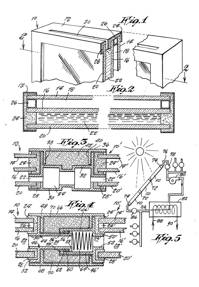
It is therefore an object of the present invention to provide an improved heat absorbing window for use in a solar energy system.
