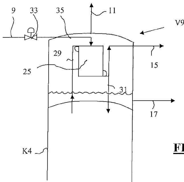
(57) Abstract : The invention relates to a cryogenic distillation separation column (K4) for separating a mixture including, as main components, carbon monoxide and either methane or nitrogen, wherein said column includes a head condenser (V9) comprising a film vaporiser (25).
