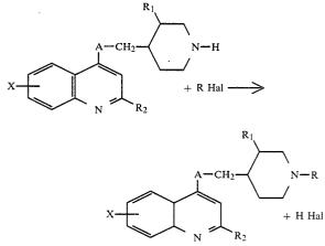
The alkylation reaction of the compounds of formula (I) for which R = H by means of an alkylating agent is effected according to processes known in the art, such as those described by R. B. WAGNER and H. D. ZOOK (Synthetic Organic Chemistry, p. 666, J. WILEY and Sons, 1965). The operation is advantageously effected in the presence of an organic or mineral base (for example sodium or potassium carbonate), in an inert solvent, for example dimethylformamide.
